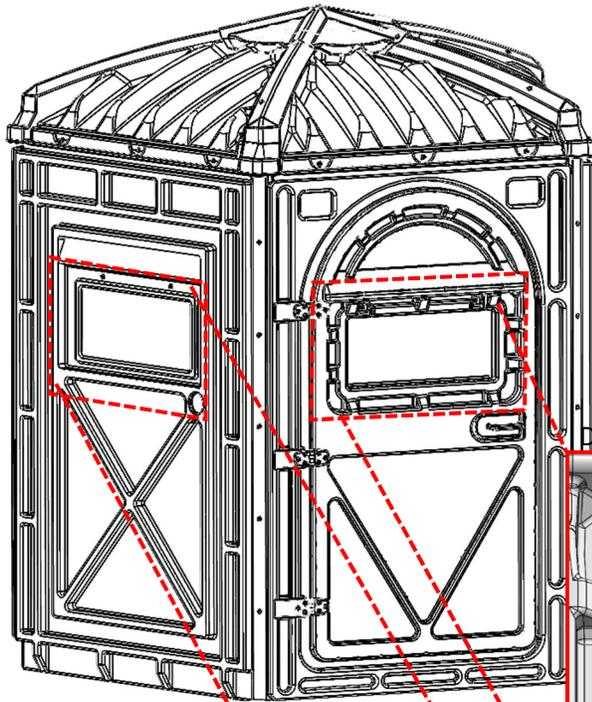
**STEP 11:** Install (10) Window Latches [INS-TERRAIN-TURN-BUTTON] into the Door/Frame Assembly [04627V-A] and (4) Common Sidewall Panels [03864V-A]. Use (10) Bolts (10-32 X 3/4") [2023] and (10) Nuts (10-32 Lock Nut) [6014].
