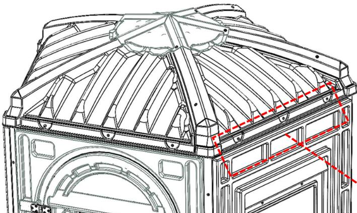
**STEP 7:** Align the Range Roof Assembly above the wall and door panels so that the holes overlap each other. Fasten the Range Roof assembly to the door/wall assembly with (5) Bolt ¼-20 x 1-¼" [2020], (5) Washer ¼ ID ½ OD [3014], and (5) Wing Nut ¼-20 [6013]. Fasten through the middle hole on each roof panel and the slots on the wall/door panels.
