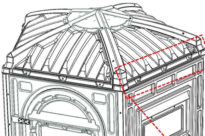
**STEP 8:** Finish fastening the Range Roof assembly to the assembly with (10) Bolt ¼-20 x 1-¼" [2020], (10) Washer ¼ ID ½ OD [3014], and (10) Wing Nut ¼-20 [6013]. Fasten through the two outer holes on each roof panel and the slots on the wall/door panels.
