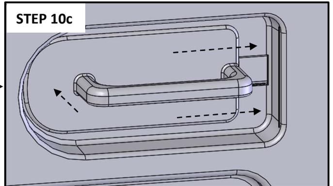
**STEP 10c:** While applying pressure in on the handle to keep the tabs in the slot, slide the handle towards the door frame.
