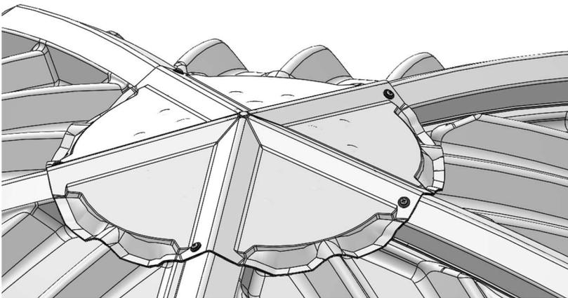
**STEP 6:** Locate the Range Roof Cap [04630V] and align the roof cap over the center of the roof assembly. The roof assembly will be required to be standing on its side. Then attach the roof cap with (5) Bolt ¼-20 x 1-¼" [2020], (5) Washer (¼ID Rubber) [3013], and (5) Wing Nut ¼-20 [6013]. Once the bolts are in place, tighten down.
