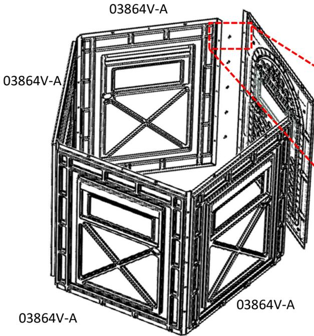
**STEP 3:** Attach (1) Door/Frame Assembly [004627V-A] panels to the assembly using (5) Bolt ¼-20 x 1-¼" [2020], (5) Washer ¼ ID ⅝ OD [3014], and (5) Wing Nut ¼-20 [6013].
