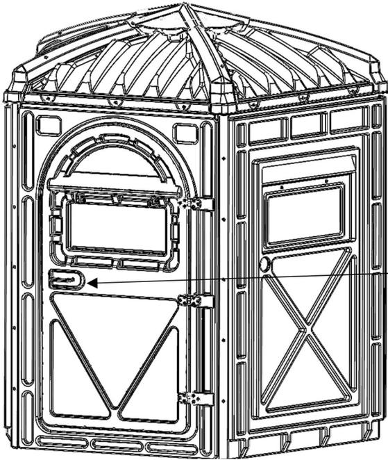
**STEP 9:** Install the Door Handle [INS-TERRAIN-HANDLE] into the Door/Frame Assembly [04627V-A] panel. This step does not require any additional hardware.
