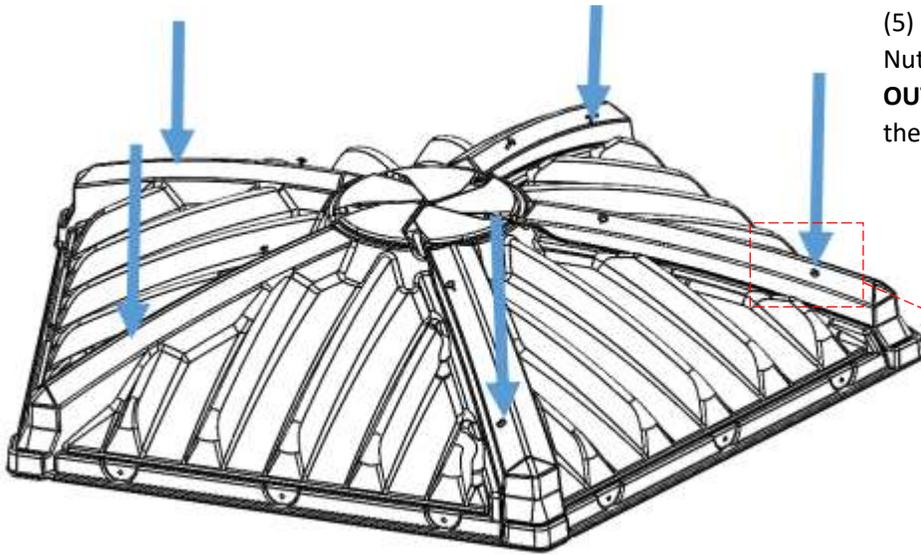
**STEP 5:** Lay each section of the (5) Range Roof Panel [03866V-C] so they overlap each other with the holes lined up, small ribs inside the large ribs. Fasten the (5) Range Roof Panels to the assembly using (5) Bolt ¼-20 x 1-¼" [2020], (5) Washer (¼ID Rubber) [3013], and (5) Wing Nut ¼-20 [6013]. Fasten only through the **OUTSIDE HOLES** on each side. Do not tighten all the way.
