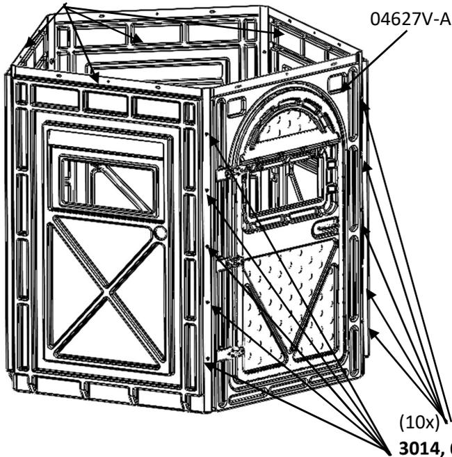
**STEP 4:** Finish fastening the Door/Frame Assembly [04627V-A] panels to the assembly using (5) Bolt ¼-20 x 1-¼" [2020], (5) Washer ¼ ID ⅝ OD [3014], and (5) Wing Nut ¼-20 [6013].
