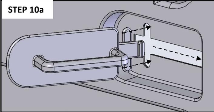
**STEP 10a:** Install the Door Handle [INS-TERRAIN-HANDLE] into the Door/Frame Assembly [04627V-A] from the exterior of the panel. Insert the tabs near the latch on the Door Handle into the slot as shown. Slide the partially installed handle towards the door frame.
