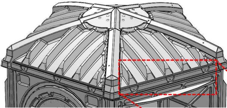
**STEP 8:** Finish fastening the Roof to the assembly with (8) Bolt ¼-20 x 7/8" [2022], (8) Washer ¼ ID ¾ OD [3014], and (8) Wing Nut ¼-20 [6013]. Fasten through the holes on the Roof and the slots on the wall/door panels.
