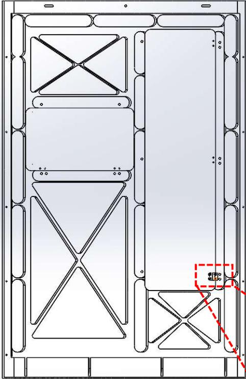
**STEP 12a:** Using 2 bolts (2021), a hinge, and 2 nuts (6012) attach the hinge to the long window as shown (RED IN PHOTO BELOW). Using 2 more bolts (2021) and 2 nuts (6012) attach the hinge to the blind wall (BLACK IN PHOTO BELOW). Make sure the nuts are on the outside of the blind wall and window as shown.
