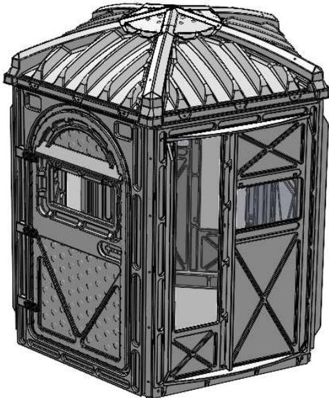
**STEP 9:** Install the Door Handle [INS-TERRAIN-HANDLE] into the Door/Frame Assembly [04627V-A] panel. This step does not require any additional hardware.
