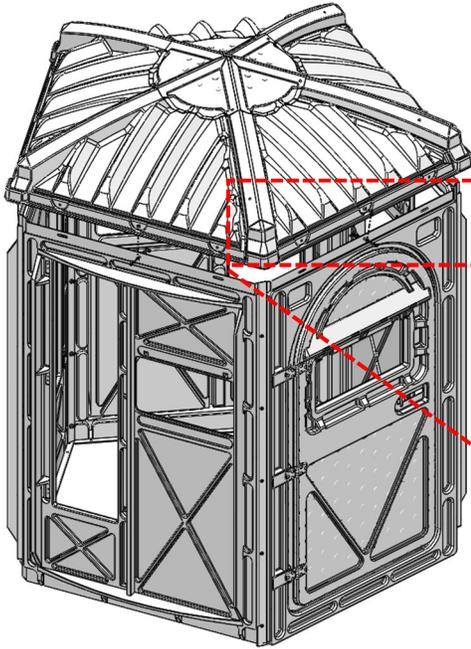
**STEP 7:** Fasten the Roof to the assembly using (4) Bolt  $\frac{1}{4}$ -20 x  $\frac{7}{8}$ " [2022], (4) Washer  $\frac{1}{4}$  ID  $\frac{5}{8}$  OD [3014], and (4) Wing Nut  $\frac{1}{4}$ -20 [6013]. Fasten only through the **MIDDLE HOLES** on each side.
