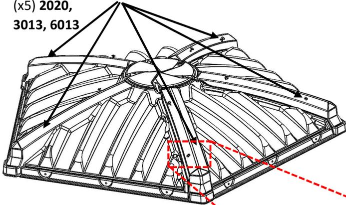
**STEP 5:** Locate all 5 roof sections [3866V-C]. Lay each section so they overlap each other with the holes lined up, small ribs inside large ribs. Using a Phillips screw driver, attach the roof section together at the Outside holes only, using the 2022 bolts provided, the rubber washers, and the wingnuts. Do not tighten all the way.
